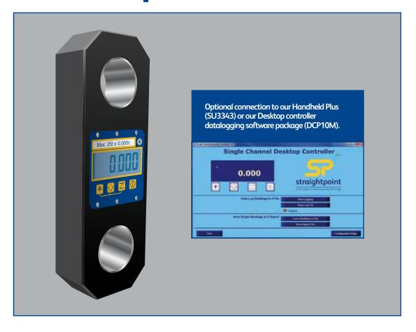
Known worldwide as the original electronic force measurement device to feature an integral display, the Loadlink Plus has been in production since 1979. Over the years the line has been expanded and the Loadlink Plus is now used on a daily basis for load monitoring and heavy lifts ranging in capacity from 1t - 500t, by a variety of industrial and commercial industries to include manufacturing, transportation, agriculture, oil and gas, utilities, aerospace and clean energy.
