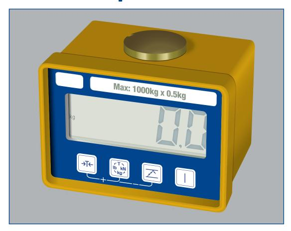
The Loadblock Plus is a low capacity, self-indicating compression load cell, used in many testing and load monitoring applications worldwide. The integral display eliminates the need for a separate display or cable assemble that can be easily damaged. Applications include the measurement of loads associated with the testing of hydraulic presses, cylinders or jacks.
