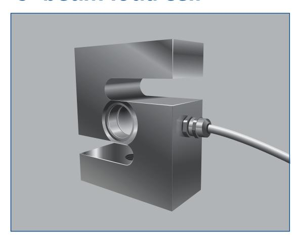
A range of stainless steel 'S' beam load cells from 1100lbs to 11,000lbs. The Straightpoint 'S' Beam range of tension/compression load cells are suitable for smaller Silo, vessel and tank weighing applications or for building into OEM projects, testing machines etc.
