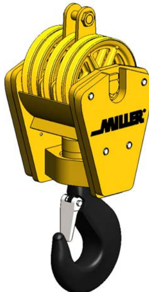
MODEL NO: 520H80 -5 SHEAVES, 20" DIAMETER -CHEEK WEIGHTS -80 TON WLL
