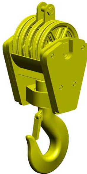
MODEL NO: 520H80 -5 SHEAVES, 20" DIAMETER -CHEEK WEIGHTS -80 TON WLL
