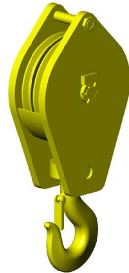
MODEL NO: 224T50 -2 SHEAVES, 24" DIAMETER -EXTENDED SIDE PLATES -50 TON WLL
